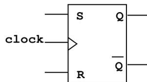
$$Q_{t+1} = S\overline{R} + Q_t\overline{S}\overline{R} = \overline{R}(S + Q_t\overline{S}) = \overline{R}(S + \overline{S})(S + Q_t) = \overline{R}S + \overline{R}Q_t \text{ (on the edge)}$$
