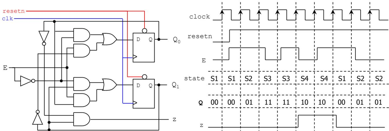
**Example:** 2-bit counter with enable and 'z' output. The output 'z' is 1 when the present count is '11'. The count is the same as the states encoded in binary.
