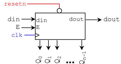
**Parallel access shift register with enable**
