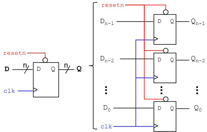
**N-BIT SHIFT REGISTER:** This is a collection of 'n' D-type flip flops, connected serially. The flip flops share the same `resetrn` and `clock` signals. The serial input is called 'din', and the serial output is called 'dout'. The flip flop outputs (also called the parallel output) are called  $Q = Q_{n-1}Q_{n-2} \dots Q_0$ . Depending on how we label the bits, we can have:
