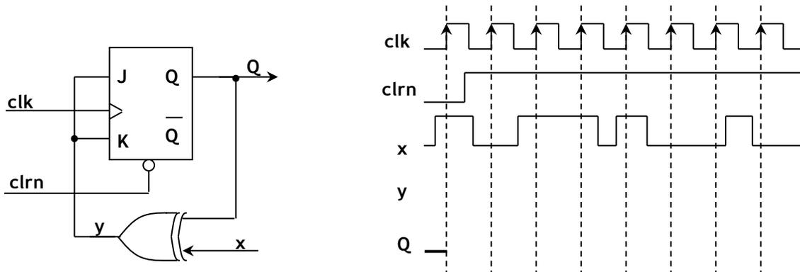
8. Complete the timing diagram of the circuit shown below:
