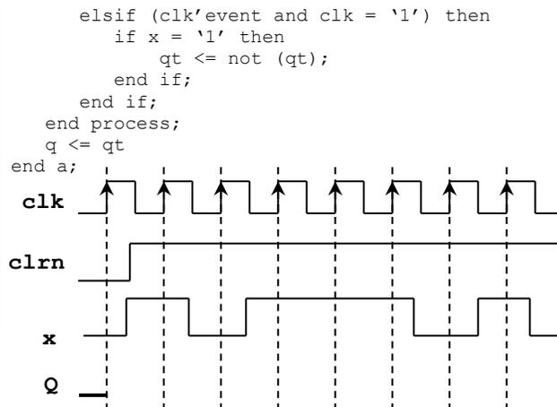
5. Complete the timing diagram of the circuit shown below:
