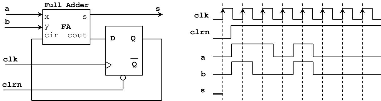
6. Complete the VHDL description of the synchronous sequential circuit whose truth table is shown below:
